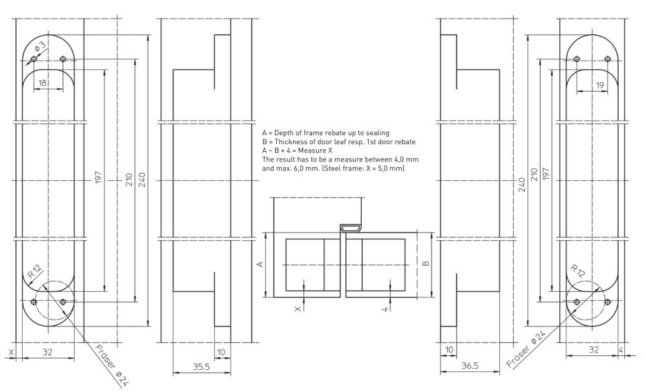
Use a 1/2" router bit with a 5/8" template guide for Templaco Router Templates
